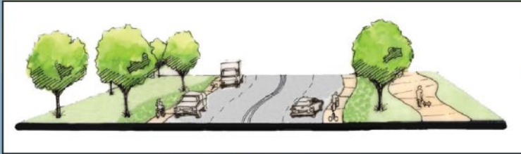
Typical Section - 4 Lane Roadway
